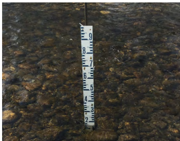
Figure 14. Streamflow measurement using a staff gauge
