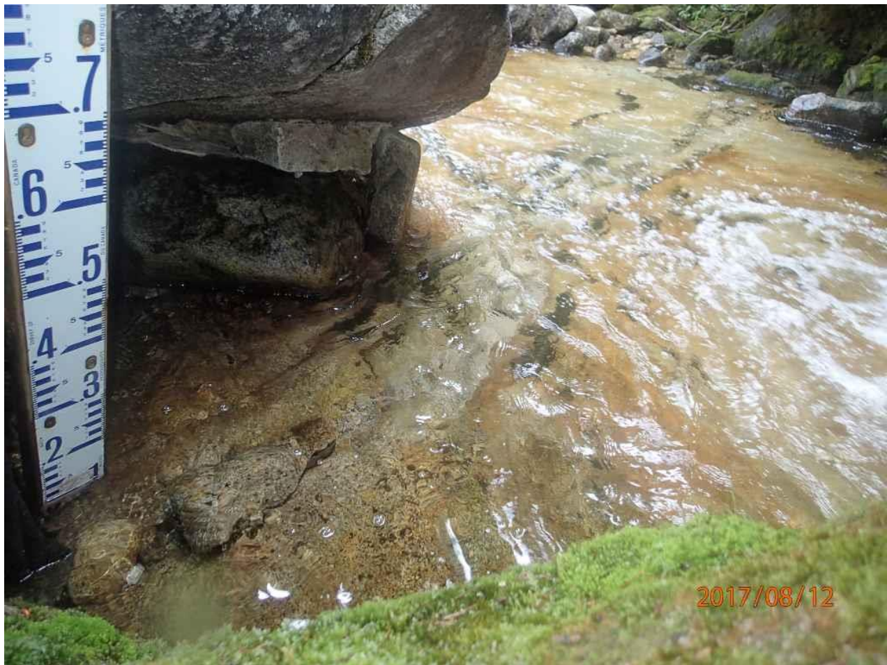
Figure 6. Photograph of staff gauge and cross section at Carlyle Creek hydrometric station.
